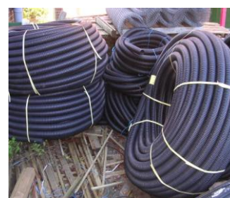
Modern drainage pipe
