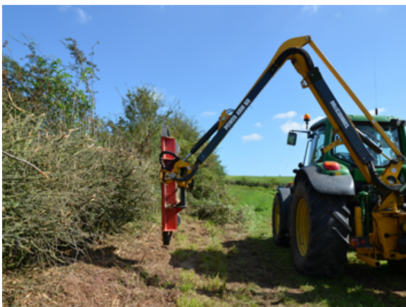
Shapesaw used for taking back heavy growth – Credit: Tony Seymour – © TFE 2014
